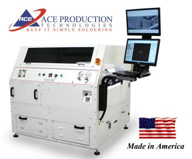
The KISS-103IL is a fully configured *In-Line SMEMA compatible* Selective Soldering Machine ready to process "LARGE" PCBs.
