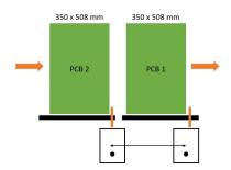
Integra 508.4 Two-Segment — soldering a panelized board with dual nozzles.
